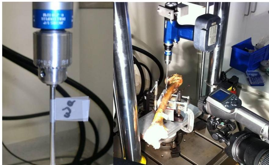
**Figure 2: Drill mounted (L) and drill test setup (R)**
