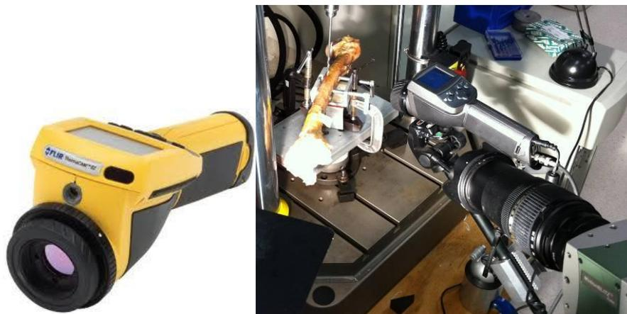
**Figure 3: FLIR IR thermal camera (L) and test setup (R)**
