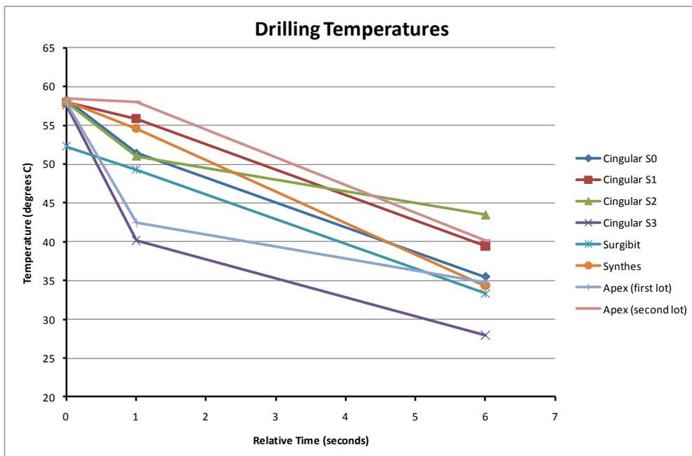
**Figure 6: CingleBit (Cingular and Apex), SurgiBit and Synthes drilling temperatures in human cortical bone**
