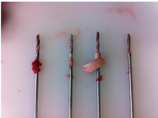
**Figure 9: Drills following soft tissue damage testing.**
