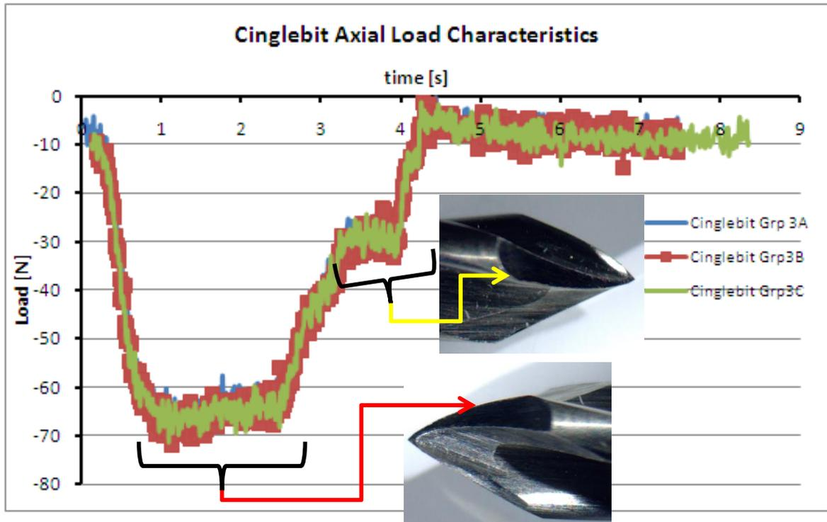
**Figure 7:** These example axial load curves for the Cinglebit show how the curve gently slopes away once the peak load has been reached; this is a characteristic of the curved cutting edge (red arrow). As the cutting edge approaches the full diameter the “brake” in the curve is due to the cutting edge “run off” to the flute (yellow arrow)
