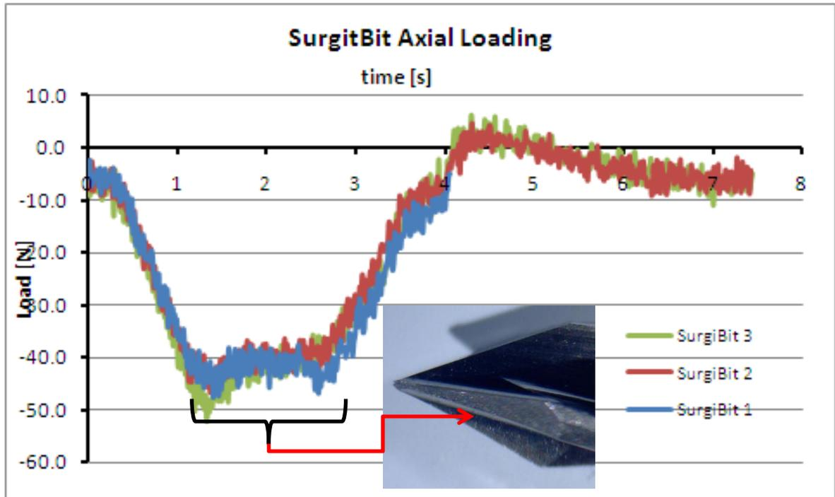
Figure 8: These example axial load curves for the SurgiBit show how the curve does not slope away as the Cinglebit does, but flattens out once the peak load has been reached; this is a characteristic of the straight cutting edge (red arrow). There is no “brake” prior to the cutting edge reaching the flute.
