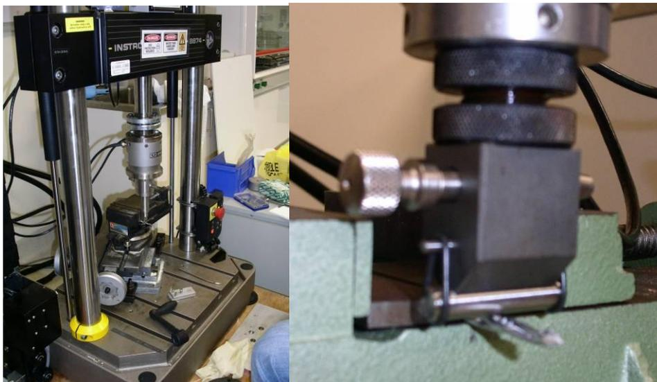
**Figure 4: Cantilever bending**
