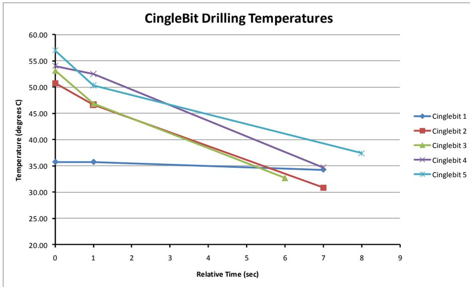
**Figure 5: CingleBit drilling temperatures in human cortical bone**
