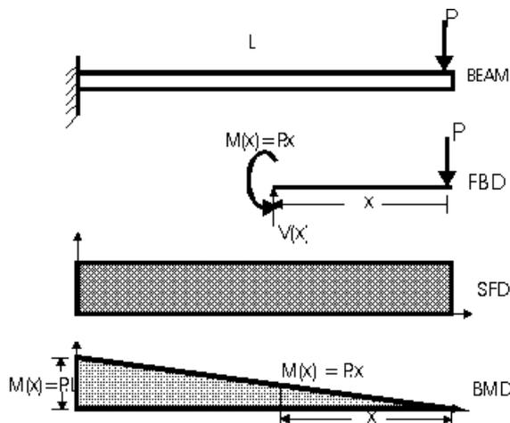
**Figure 10: Schematic showing a bending moment diagram (BMC). In the bending test,  $L=10\text{mm}$  and  $P$  was applied at  $2\text{mm/s}$ . And  $M_{\text{Max}}=P_{\text{Peak}}L$**
